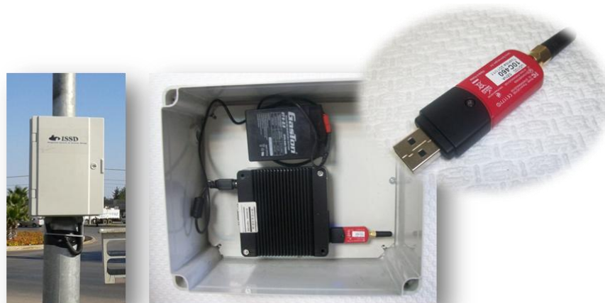
Figure 3 Class 1 type Bluetooth reader device with antenna (range 300m) used in the Etlik study
